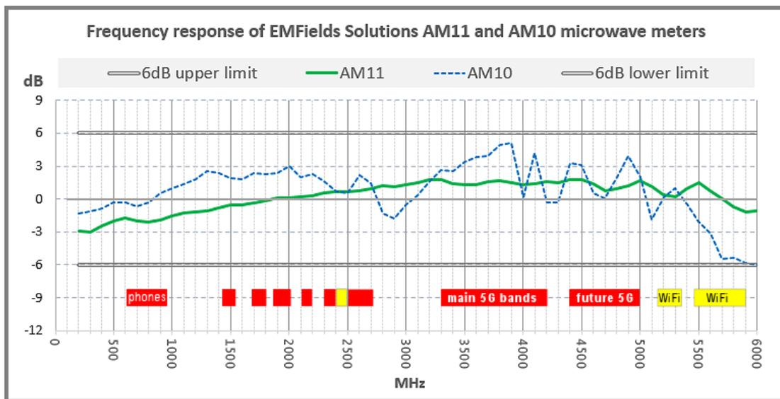
As the graph shows, the AM11 has a very consistent input frequency response, and we are proud of the accuracy we have been able to achieve. It is worth noting that to be within  $\pm 6$ dB is considered to be good accuracy when measuring microwave EMFs with a broad-band microwave meter. The AM11 response extends to 8 GHz. As a comparison, we show, below, an example of another other competitor instrument (name withheld) measured using the same test set-up and technique.
